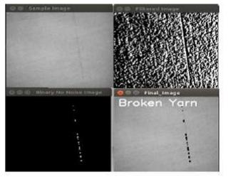
Fig. (8) Result of Type Defect (Broken Yarn/Needle)
